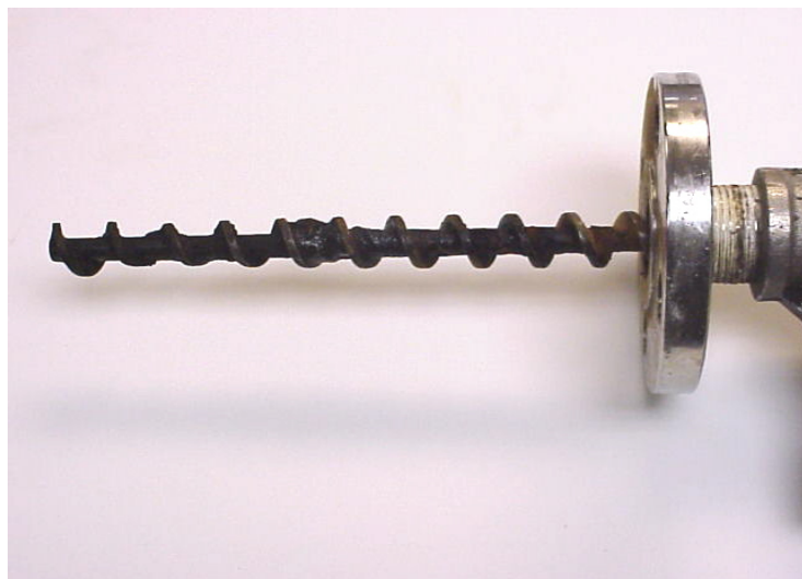
Figure 10. Auger feeder with ALM lignin plug formed between flights
