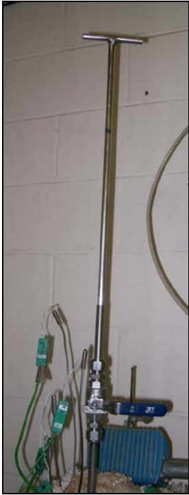
Figure 4. Single valve with push rod
