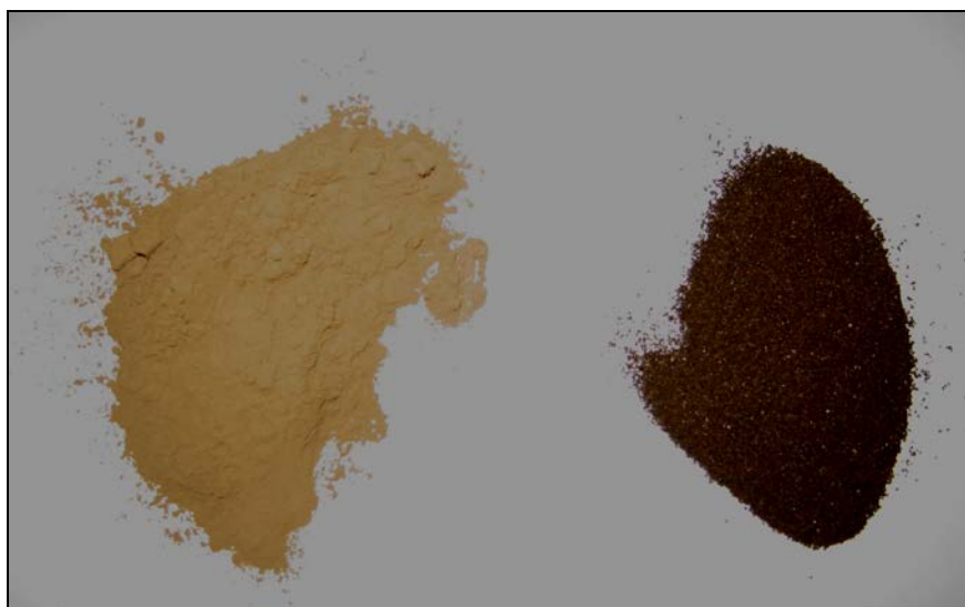
Figure 5. ALM lignin before pre-treatment (<100 microns) (left) and after pre-treatment (355 to 1000 microns) (right)
